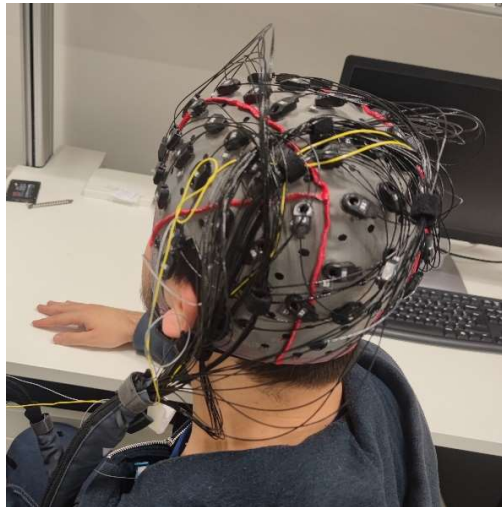
Fig. 1: EEG cap used for the experiment.
