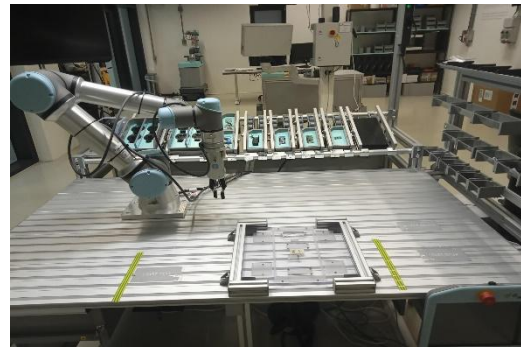
Fig. 2: Collaborative assembly station with UR5e robot
